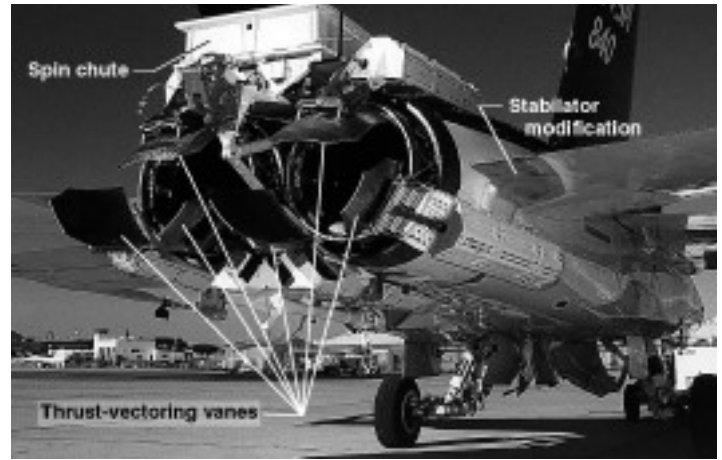
Thrust-vectoring control system. (NASA photo EC90-177-4 with text added)
