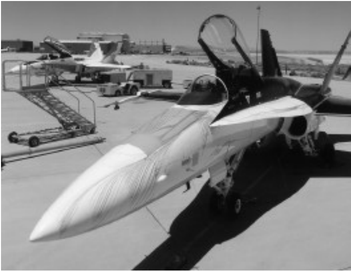
Dye from small holes in the nose of the F-18 HARV showing the flow of air. (NASA photo EC88-0015-79)
