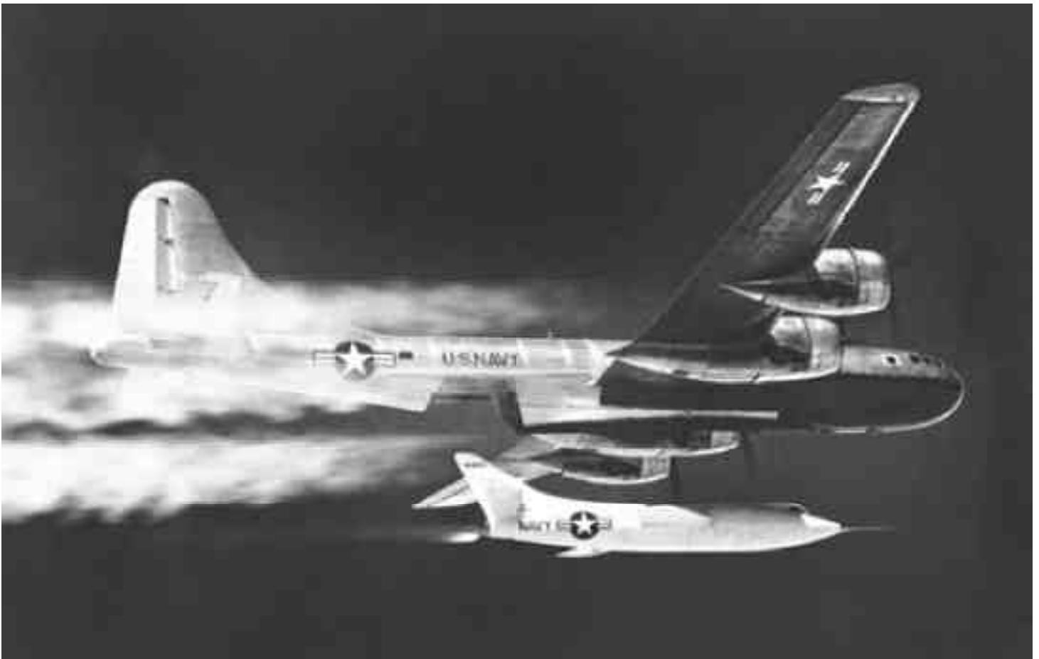
D-558-II Skyrocket being launched from a P2B.
