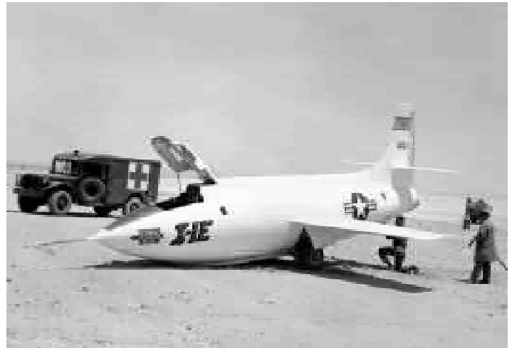
Photo E-2369. X-1E on lakebed with collapsed nose gear.
