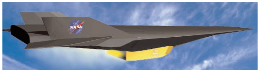
The Hyper-X program has significantly expanded the boundaries of air-breathing flight by being the first to fly a "scramjet" powered aircraft at hypersonic speeds.
