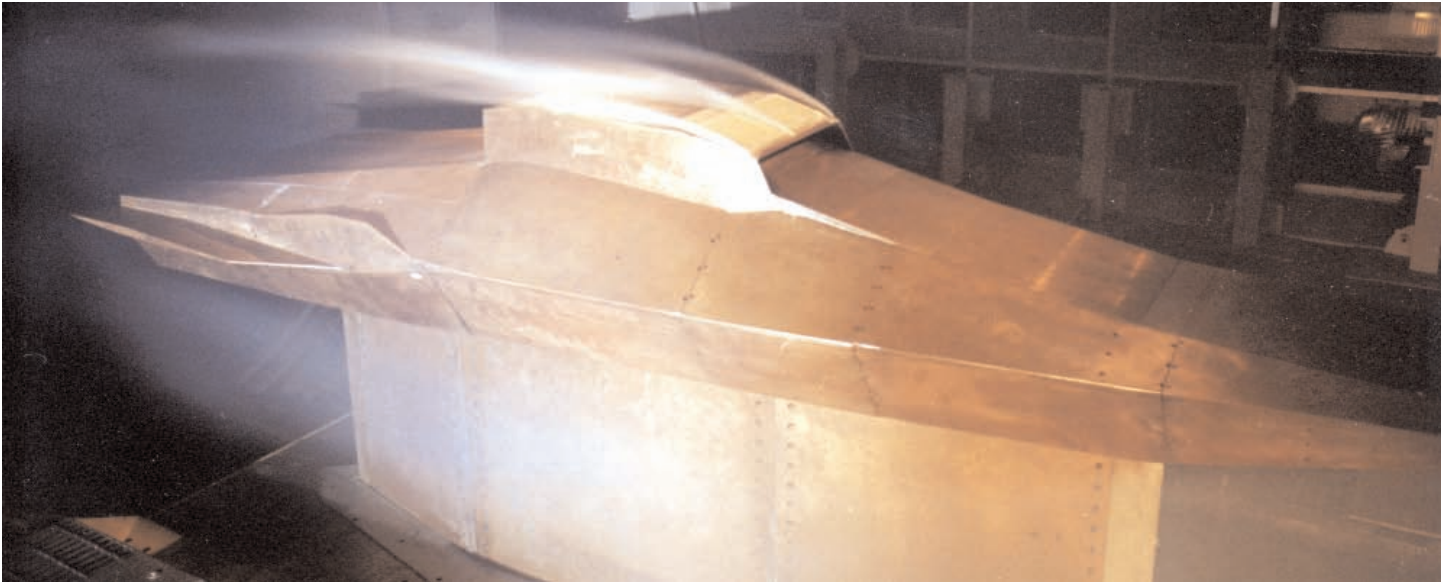
Wind tunnel tests were a necessary step before the first flight attempt, as in this Mach 7 test of a full-scale model with spare flight engine in Langley's 8-Foot High Temperature Tunnel.
