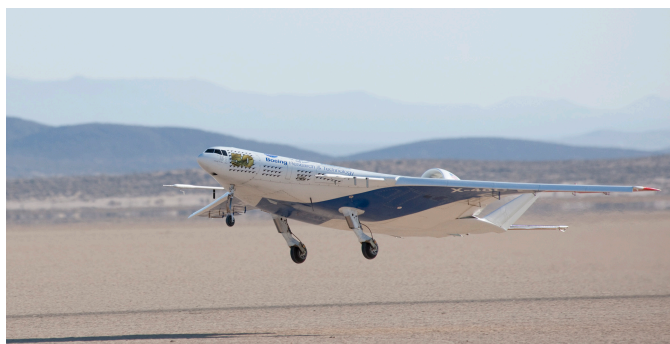
The remotely operated X-48C Blended Wing Body aircraft lifts off Rogers Dry Lake at Edwards Air Force Base, Calif., on its first test flight Aug. 7, 2012. (NASA / Carla Thomas)
