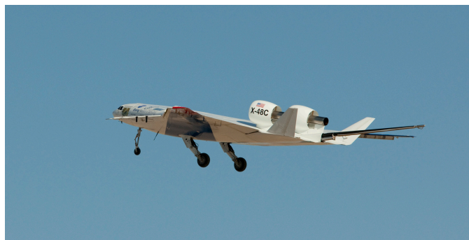
The X-48C Hybrid / Blended Wing Body technology demonstrator lifts into the skies after taking off from the bed of Rogers Dry Lake at Edwards Air Force Base on its first test flight. (NASA / Carla Thomas)
