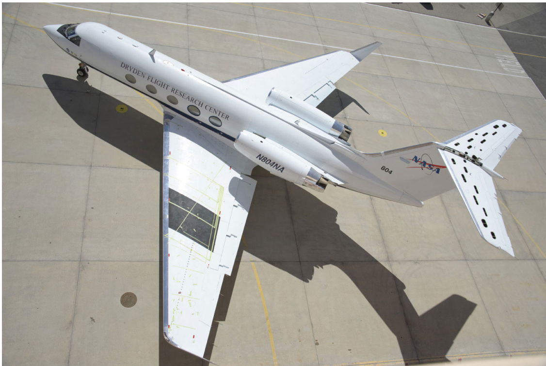
The Active Compliant Trailing Edge (ACTE) project will replace both of the G-III's conventional 19-foot-long aluminum flaps with advanced, shape-changing composite-material flaps that form continuous bendable surfaces. (NASA / Tony Landis)
