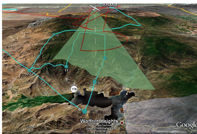
This 3-D image shows the flight track of NASA's Ikhana remotely piloted aircraft over Southern California's Lake Isabella on Nov. 19, 2009. The green swath below the Ikhana graphic depicts the scanning profile of NASA's Autonomous Modular Sensor, which operates like a digital camera with specialized filters to detect light energy at visible, infrared and thermal wavelengths. (NASA Image)
