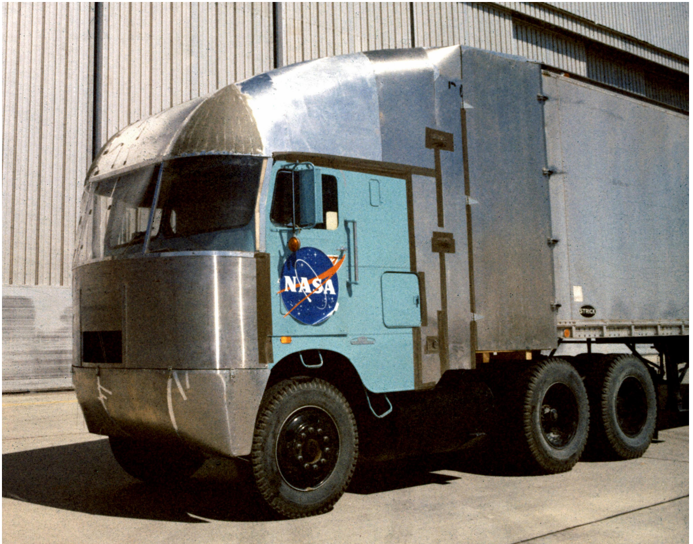
Application of aerodynamic design principles to the design of large truck cabs by NASA Dryden researchers in the mid-1970s led to the adoption of those standards by most manufacturers of large trucks on the road today. (NASA Photo)
