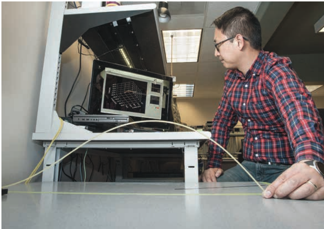
Patrick Chan demonstrates one way that the Fiber Optic Sensing System is used by bending a fiber with a 3D representation of the fiber's shape as it bends. (NASA / Ken Ulbrich)
