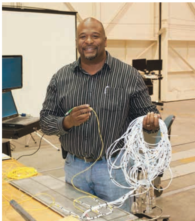
The metallic panel has conventional and fiber optic sensors. The white bundle of cables contains 100 conventional strain gages, the single yellow cable about 350. Armstrong aircraft have been used in validation of fiber optic sensors. (NASA / Tony Landis)
