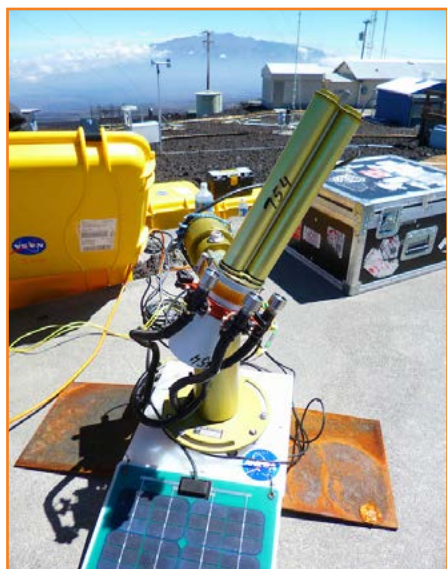
✦ Mini-LHR (as add-on to an AERONET Sun photometer), enables simultaneous monitoring of aerosols and carbon cycle gases.
