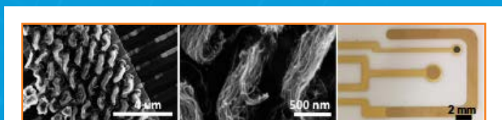
✦ Scanning electron and light microscope images of carbon nanoelectrode array. Left and center: Array of carbon nanotube electrodes. Right: Sensor device with gold working electrode.
