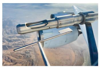
NASA's DC-8 flew in support of the NASA Student Airborne Research Project (SARP) to measure aerosols using the Langley Aerosol Research Group Experiment (LARGE) instrument with the Cavity Attenuated Phase Shift (CAPS) PMex Monitor (Particle Optical Extinction). NASA/Carla Thomas
