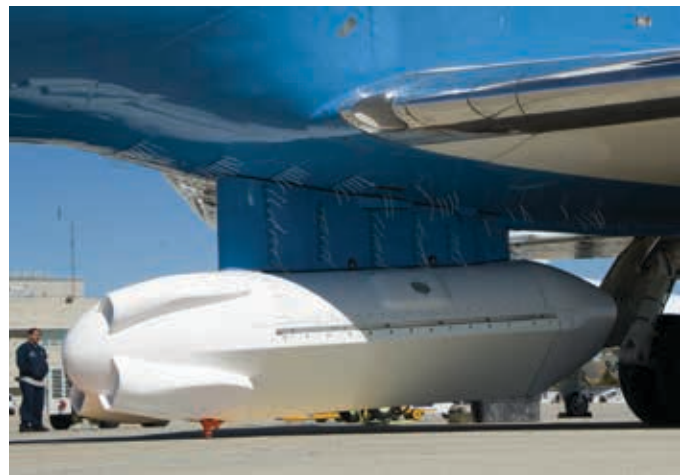
A forest of tufts are mounted on the underbelly and pylon of NASA's Gulfstream-III research aircraft to help engineers determine airflow around the UAVSAR pod. (NASA)
