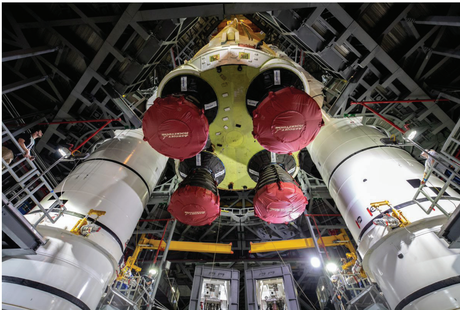
The SLS Artemis I core stage is lowered into position on the mobile launcher between the solid rocket boosters at the VAB.
