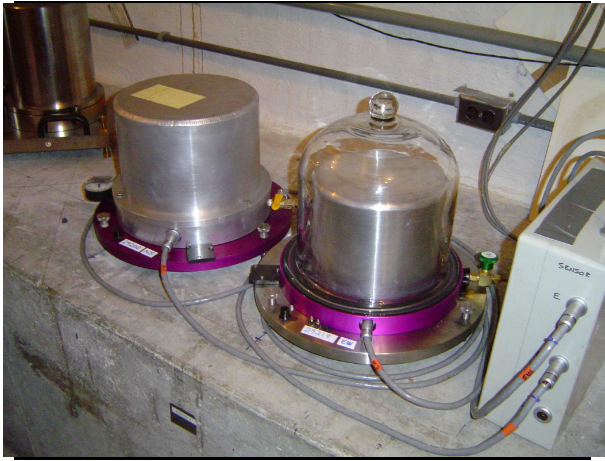
Figure 3.31: STS-1 seismometers in the Byerly Vault installed in a new pressure vessel (left) and on a warplless baseplate with a glass bell (right).
