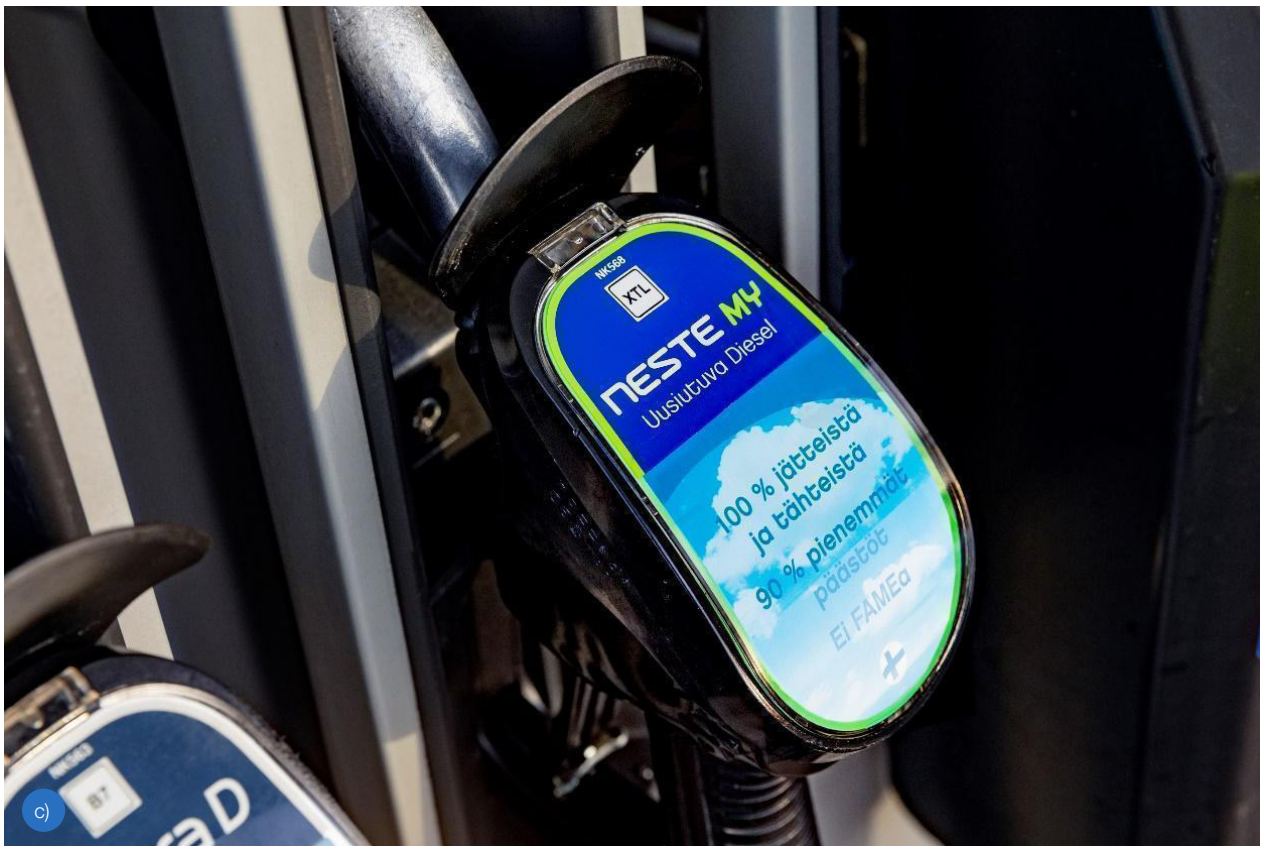
Figure 3. Examples of fuel labelling according to EN 16942 a) – b) in fuel tanks of trucks and c) in dispensers and pistols at retail points. “XTL” in the vehicle means that paraffinic diesel including renewable diesel fuel is formally accepted.
