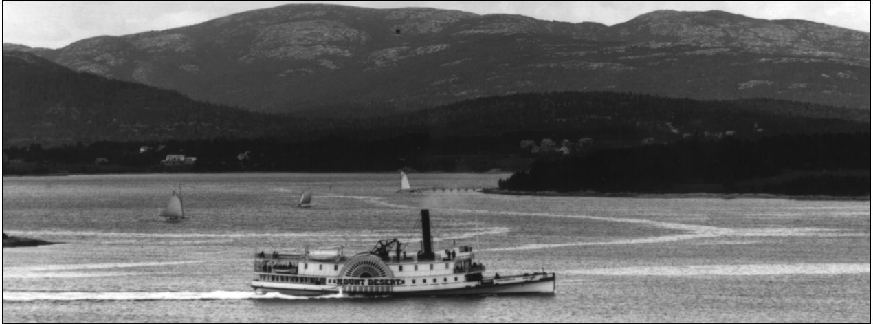
Steamer “Mt. Desert” leaving Southwest Harbor, c1900. Built by Goss & Sawyer Co. at Bath, Maine, 1879, for the Rockland, Mount Desert, & Sullivan Steamboat Co. Known as “Old Mountry,” it traveled between Rockland and Bar Harbor, stopping at Bass Harbor, Southwest Harbor and Sullivan. It was 163’ long, with a capacity of about 150 passengers. In 1904 the J.T. Morse took over Old Mountry’s Rockland-Bar Harbor run. (See Short & Sears, p.159.) (Photo by G.A. Neal. SWH Library Collections.)
