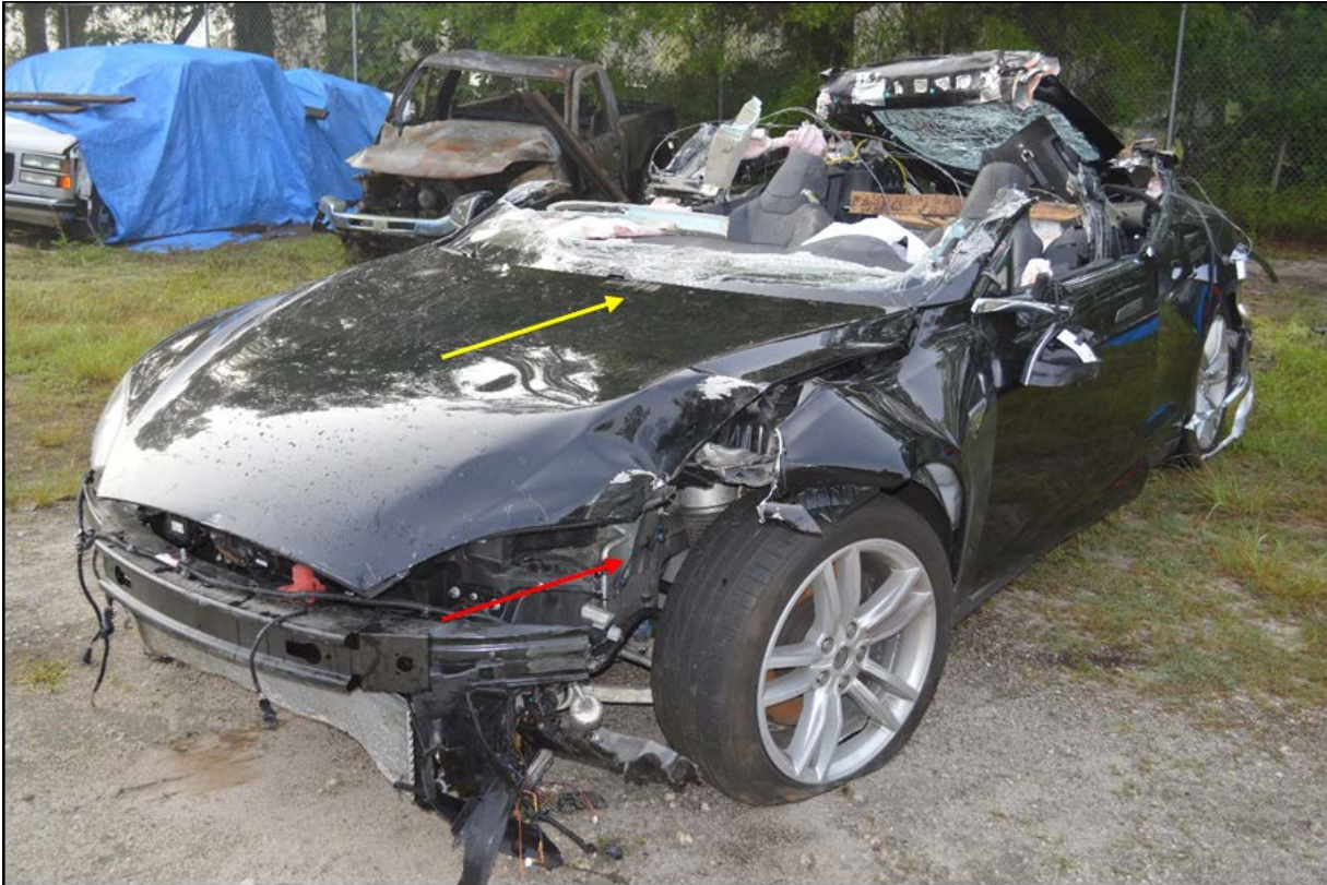
Figure 5. Damaged car. Scrapes from the semitrailer's center side-marker lamp are indicated by the yellow arrow. Impact damage associated with the utility pole is indicated by the red arrow. (Source: Florida Highway Patrol)
