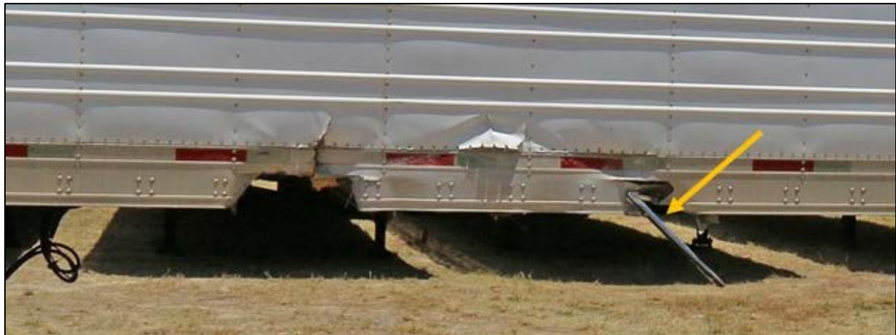
Figure 7. Closeup view of impact damage to the right side of the Utility semitrailer. The arrow indicates a segment of front windshield trim from the Tesla entangled in the forward-most area of damage.
