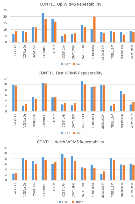
Fig. 9 WRMS position repeatability from BKG and GSFC. Apart from Hobart12M and Tsukuba Up there is good agreement.
