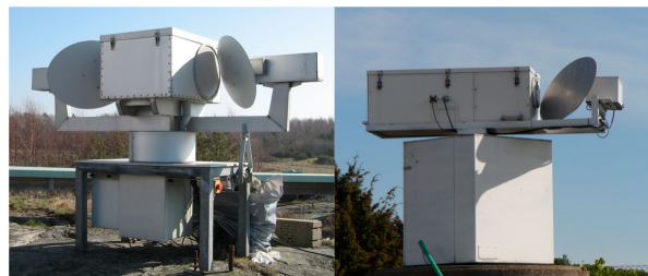
Fig. 9 The microwave radiometers Konrad (left) and Astrid (right).
