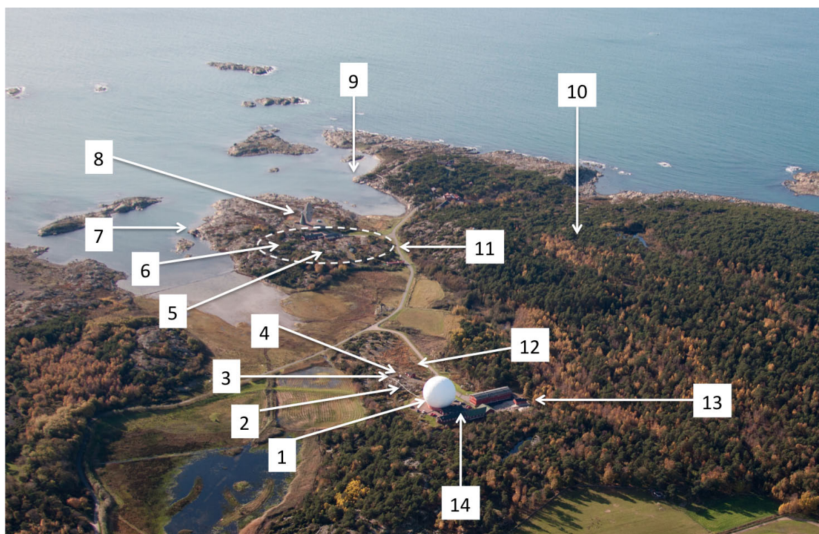
Fig. 1 Aerial photo of OSO: (1) the radome-enclosed 20 m radio telescope, (2) the microwave radiometer "Konrad", (3) the GNSS-station ONSA, (4) the microwave radiometer "Astrid", (5) the location of the northern telescope of the future Onsala Twin Telescope, (6) the location of the southern telescope of the future Onsala Twin Telescope, (7) the tide gauge station, (8) the 25 m radio telescope, (9) the GNSS-R based tide gauge, (10) the seismometer, (11) the six-station GNSS-array around the OTT, (12) the GNSS-station ONS1, (13) the gravimeter laboratory with the superconducting gravimeter, (14) the time and frequency laboratory.
