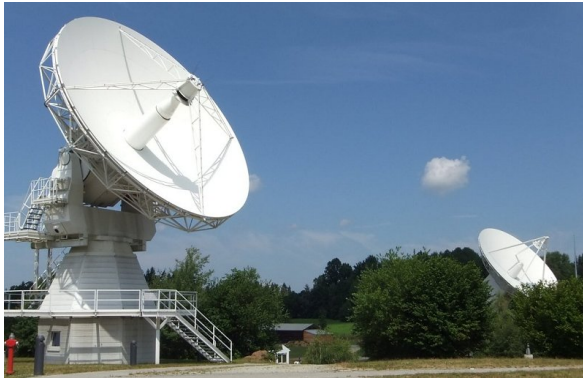
Fig. 1 Image of the 13.2 m TTW1 (left), the first of the two TWIN telescopes at Wetzell, and the 20 m RTW. The baseline between the two reference points has a length of 123 m.
