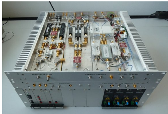
Fig. 2 Picture of the complete down-converter for the tri-band receiving system of TTW1.
