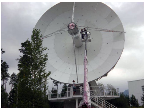
Fig. 4 Photogrammetric measurement of reflective surface.
