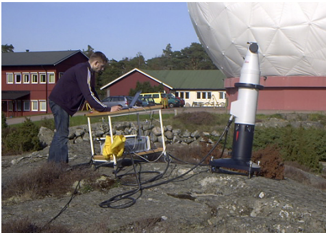
Fig. 1 Local Tie Measurement at Onsala Space Observatory with Leica Laser Tracker LTD840.
