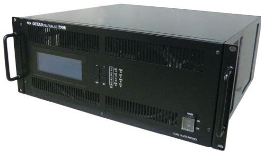
Fig. 3 The K6/Galas sampler, a direct sampling (16 GHz speed) system including DBBC signal processing.
