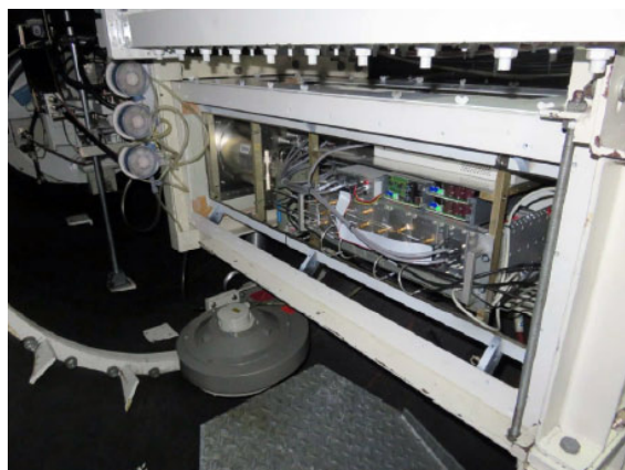
Fig. 2 New S-/X-Band VLBI Receiver at O'Higgins.
