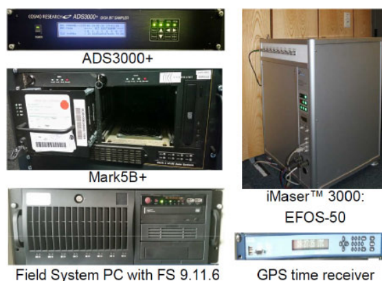
Fig. 3 Newly installed data acquisition systems for VLBI.
