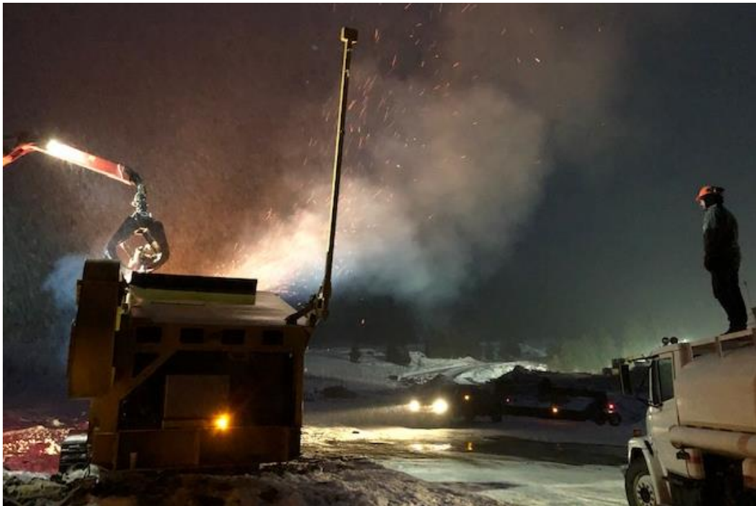
Demonstration of a new model Air Curtain Burner, "The Carbonator", showing how small-scale burning can be done near populated areas with minimal smoke impact.
