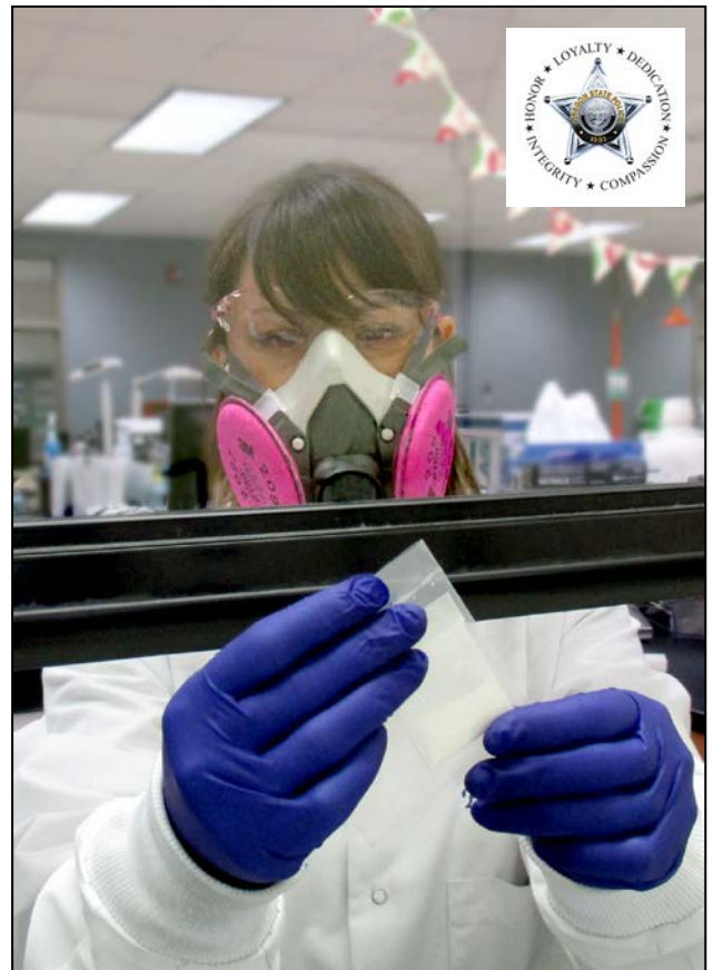
Forensic Scientist Erin Ward examines evidence suspected to contain fentanyl. She is wearing proper personal protective equipment (PPE) and working inside a ventilation hood for added protection.
