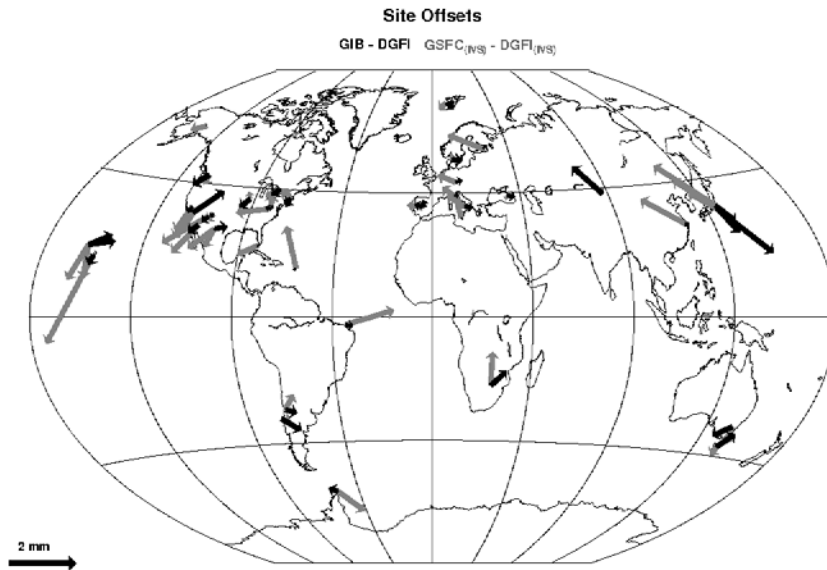
Figure 4. Horizontal offsets of all VLBI stations, GIB - DGFI differences in black, GSFC IVS and DGFI IVS differences in grey
