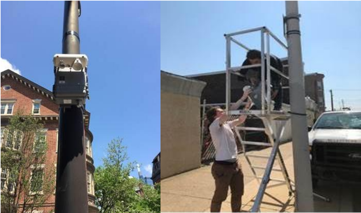
Figure 2. Sampling unit mounted on a street pole
