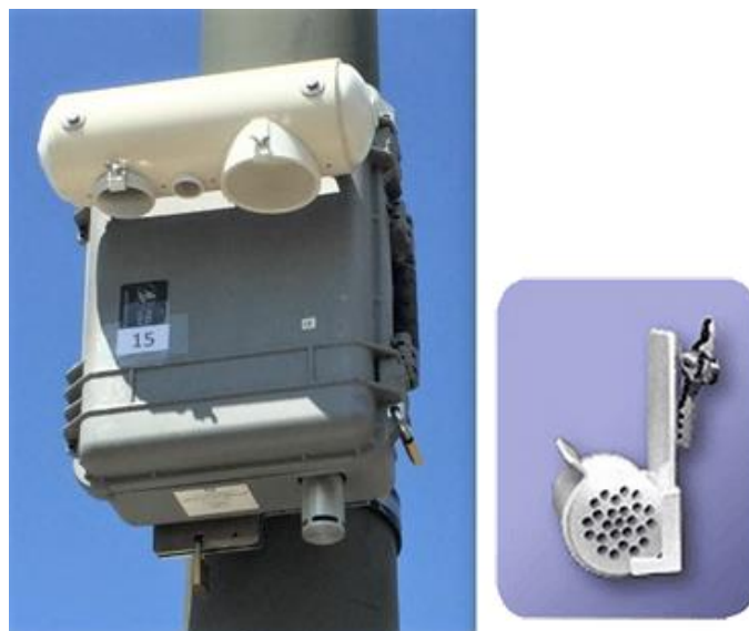
Figure 1. Multi-pollutant sampling unit (left) and passive gas sampler (right, installed in the white housing outside the sampling unit)
