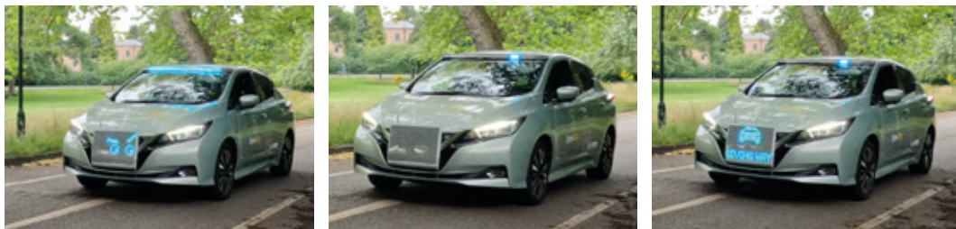
Figure 4.1: Vehicle with different eHMIs (from left to right: explicit, implicit, low anthropomorphism)
