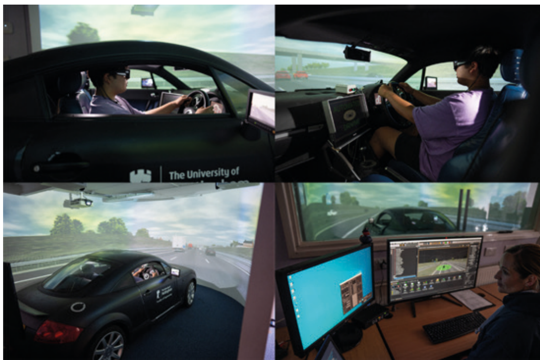
Figure 3.1: University of Nottingham’s Human Factors Research Group driving simulator, showing (clockwise from top left): side view, vehicle cabin/interior, control room and full vehicle with surrounding screen
