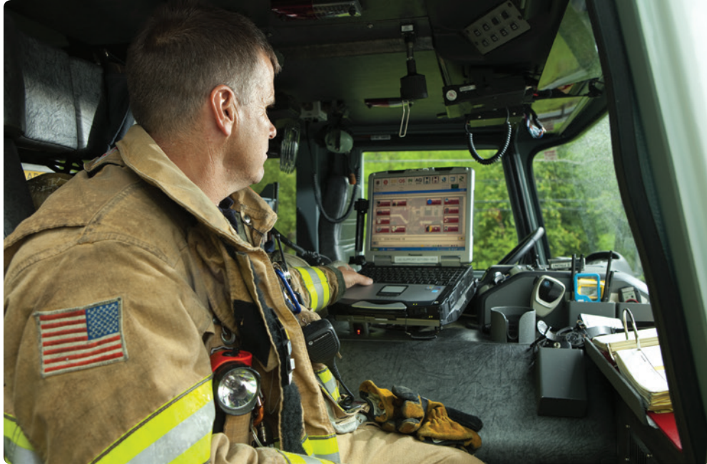
Fig. 9-1: A mobile data terminal is situated in the emergency vehicle and displays information in text that has been relayed from the base.
