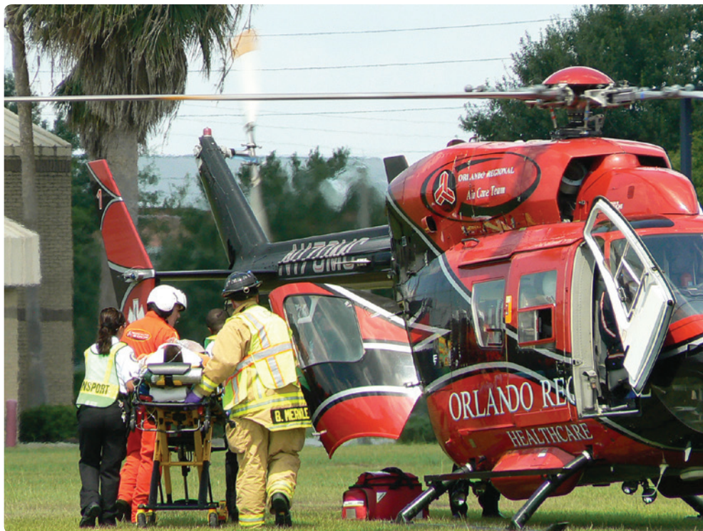
Fig. 27-10: Tail rotors are dangerous. Approach only if given permission by the pilot and only from the front or side so the pilot sees you. Photo: courtesy of Ted Crites.
