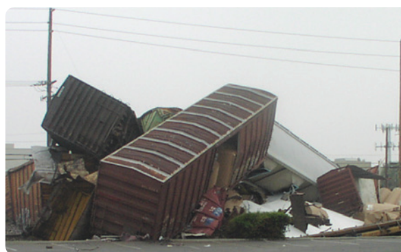
Fig. 29-4: Unusual placement or conditions and leaking containers are indications of the presence of hazardous materials. Photo: courtesy of Capt. Tony Duran, Los Angeles County Fire Department.
