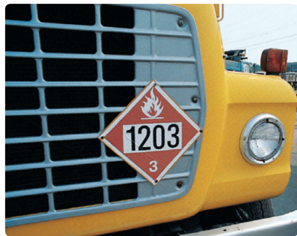
Fig. 29-5: By law, specific types of placards must indicate the presence of hazardous materials.
