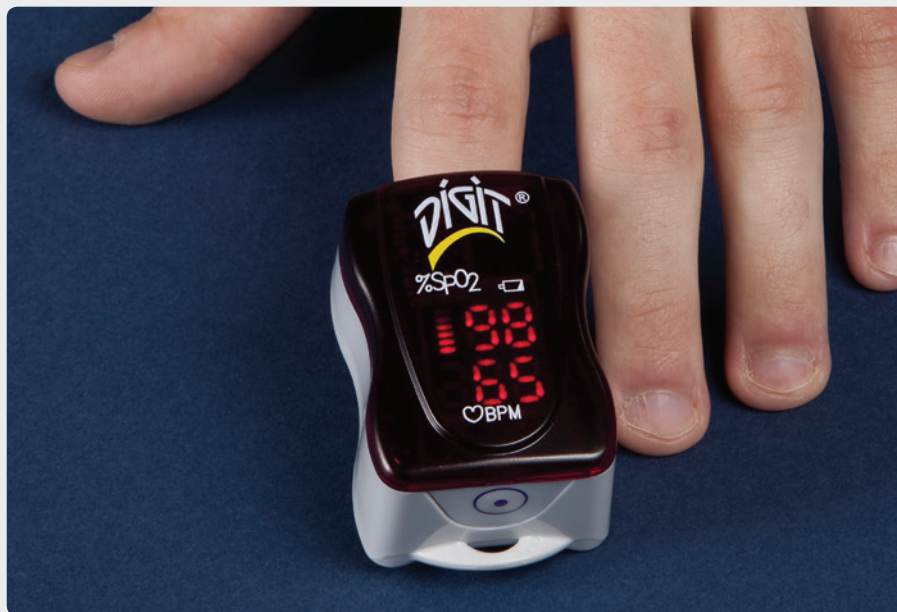
Fig. 8-19: A pulse oximeter measures the oxygen saturation level in a patient's blood.
