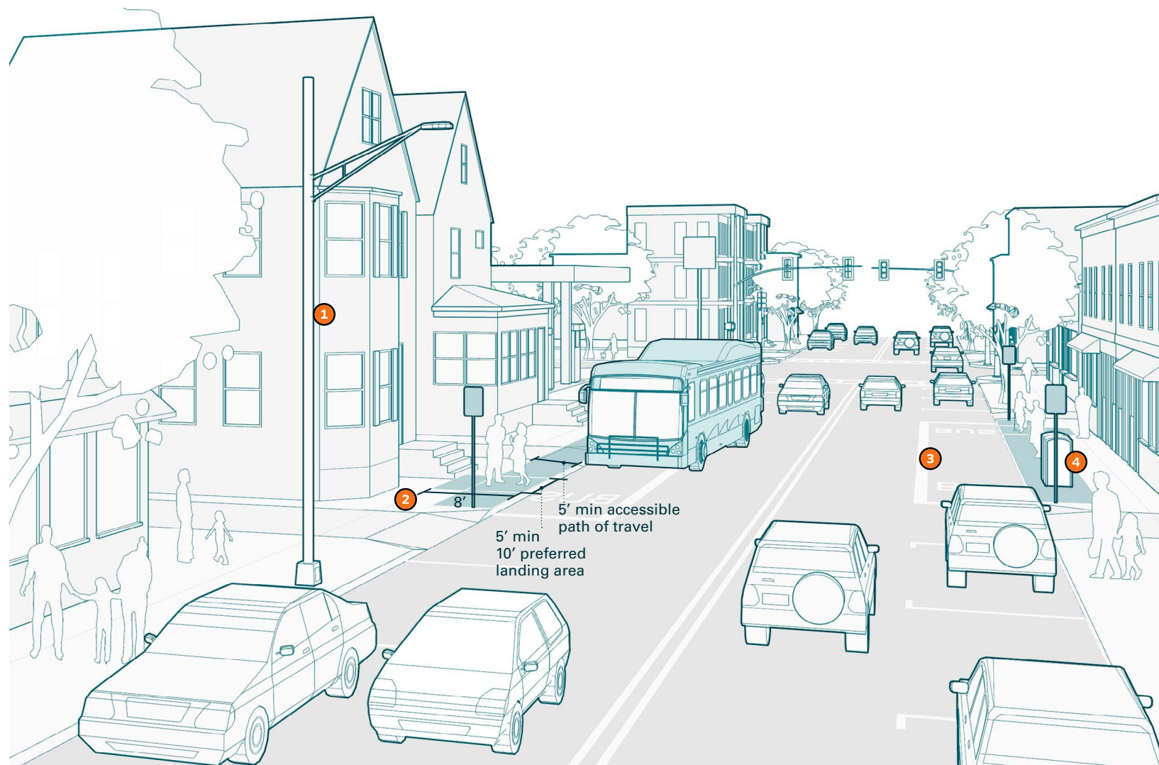
Figure 72 Bus Stop in Parking Lane with Multiple Curb-cuts
