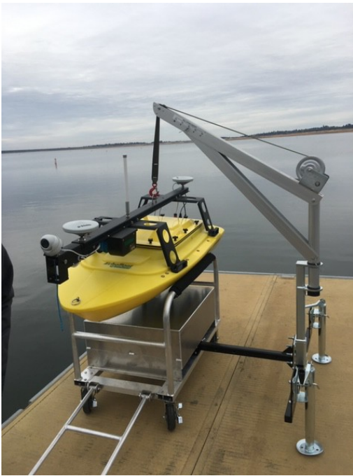
EchoBoat-160 being lowered into the water with Seafloor's EchoCart/LARS (Launch and Recovery System)
