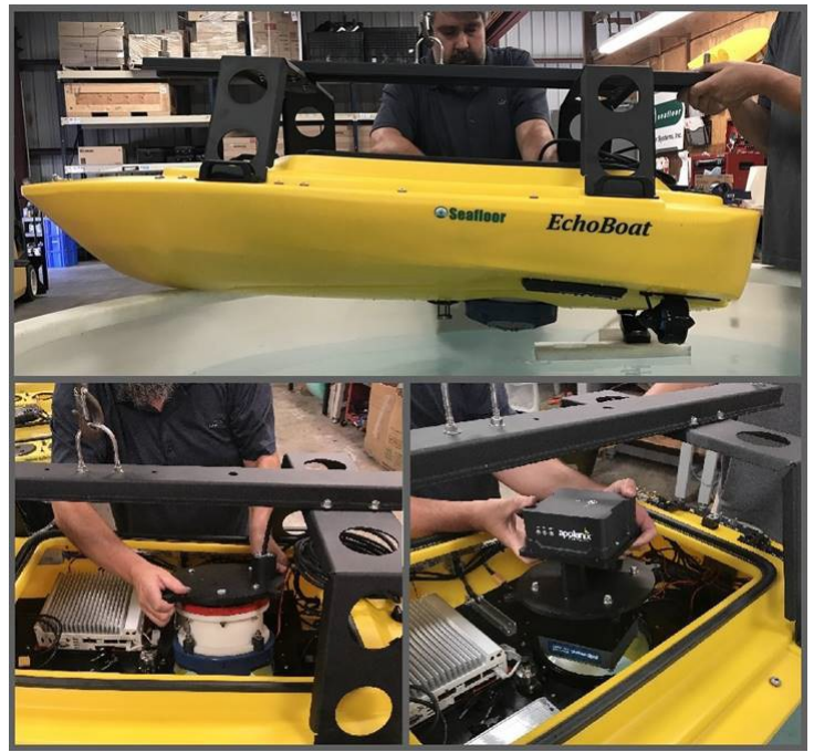
Swapping a Multibeam sonar and ADCP system in/out of the thru-hull moonpool.
