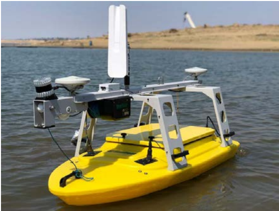
EchoBoat-160 with integrated Multibeam sonar, Inertial Navigation System, Sound velocity sensor, Sounds velocity Profiler, LIDAR scanner, and onboard PC with hydrographic survey software.
