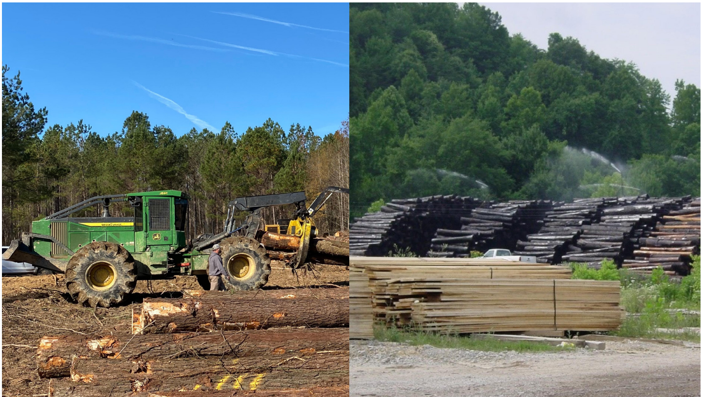
LEFT: A rubber-tired grapple skidder moving loblolly pine trees to the logging landing. (USDA Forest Service photo by William Durham); RIGHT: A stack of roundwood at the mill. (USDA Forest Service photo by Tony Johnson)
