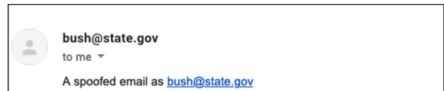
Figure 5: Example of a successful attack. A spoofed email purporting to be bush@state.gov is delivered to a Gmail user’s inbox with no warning indicators.
