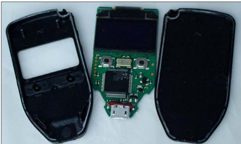
FIGURE 1 The Trezor wallet is shown here with the enclosure removed.
