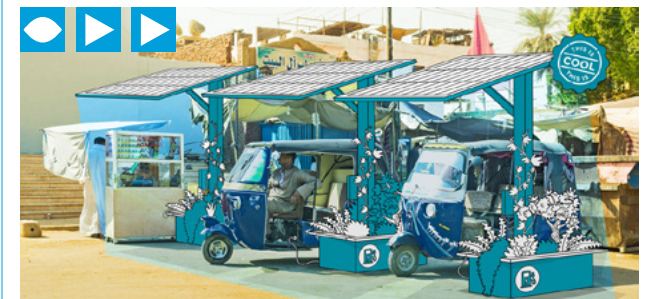
Solar roof EV charging stations provide both energy and shade. In hot, dense cities with intermittent access to electricity, this infrastructure can deliver an added secondary financial benefit as power is sold back to the grid. The Sustainable Energy for All (SEforAll) “This Is Cool” initiative shows what can be done to make sustainable cooling a reality. An SEforAll office in New York has been established to strengthen collaboration with the United Nations and drive more impactful work through UN-Energy.
