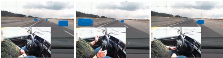
Figure 3: Sequence of driver reactions in the cases with observed collisions. Approaching obstacle with hands on lap (left), hands close to steering wheel (middle), hands put down shortly before collision (right).
