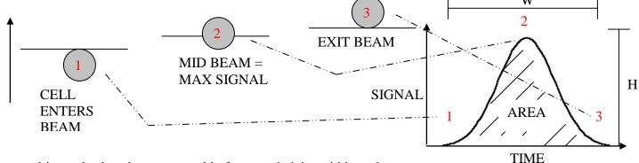
The resulting pulse has three measurable features: height, width, and area.
