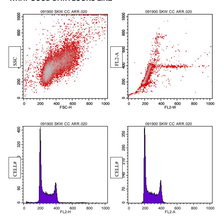
Generating data like this involves careful adjustments and readjustments of PMT voltage and Amp gain settings.
