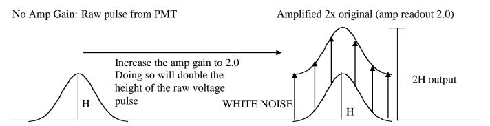
The amp gain on a flow cytometer ranges from 1.00 (no alteration of raw voltage pulse) to 9.99 (nearly 10 times the amplification). On FSC, if you need to amplify more than 9.99, you adjust the rough voltage setting to the next step (a ten-fold increase) and bring your FSC Amp gain setting back down to 1.00 – and then adjust your amp gain as necessary.
