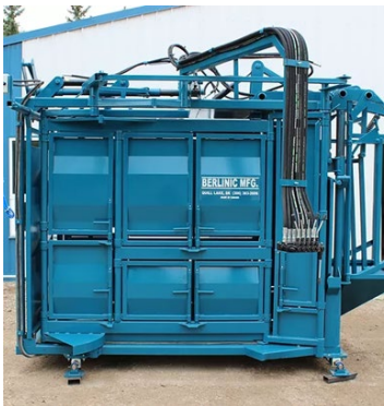
Figure 1. Example of squeeze chutes designed for buffalo management.
