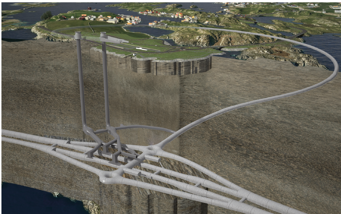
Figure 2-2. Illustration of access tunnel on Kvitsøy, distribution zone, ventilation towers, and motorway tunnels, ref. /1/.
