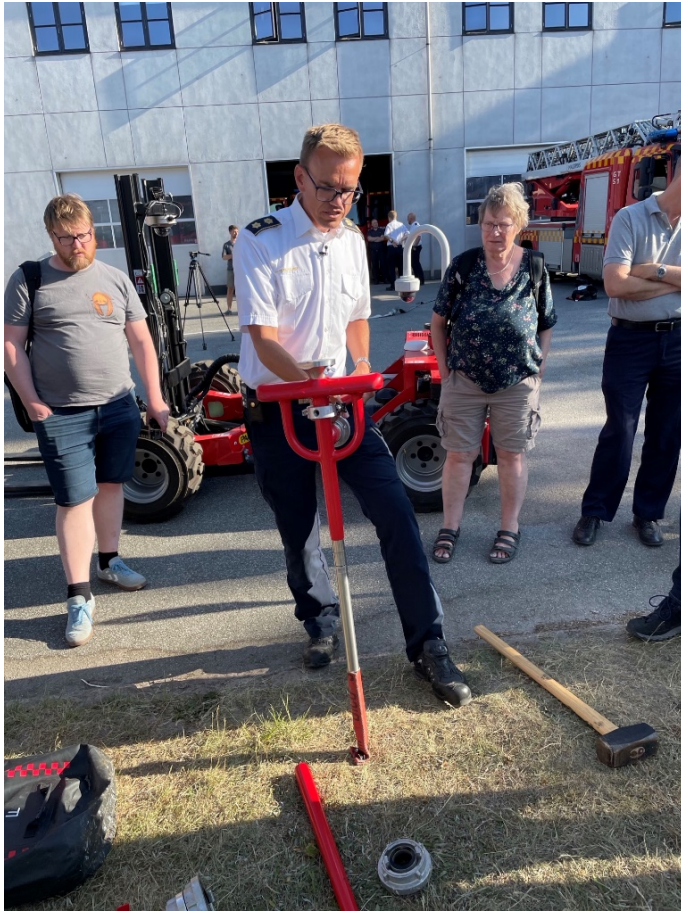
Figure 2-13 Demonstration of use of spears to flood the battery (private photo).
