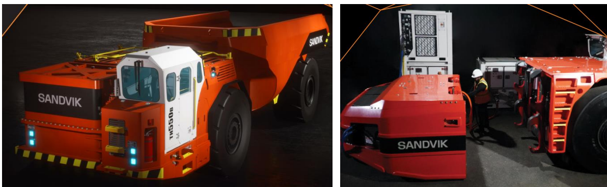
Figure 4-4: Sandvik battery-electric 50 ton ADT [42] (left) and example of the battery offloading mechanism at the recharging station [44] (right)
