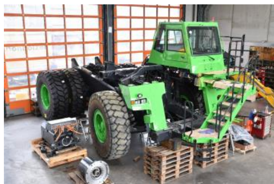
Figure 4-6: Kuhn / eMining prototype of a retrofitted Komatsu HD605-7 to battery-electric drive [52]
