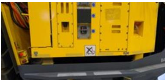
Figure 3-11: Fire hose connection on an electric construction vehicle (source: Epiroc)
