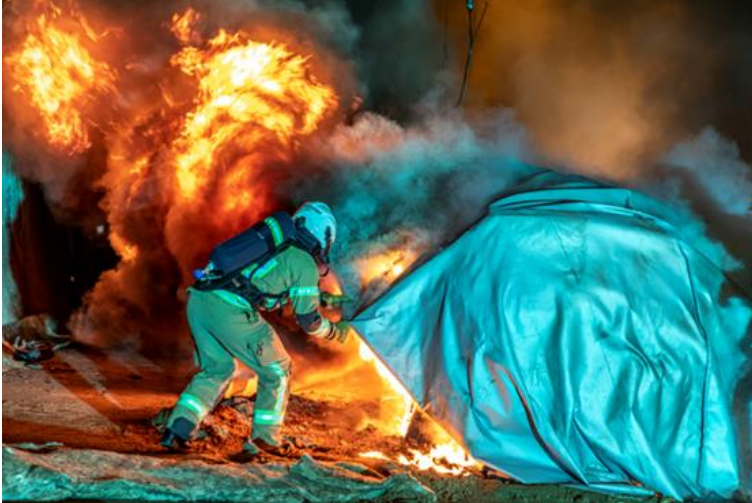
Figure 3-8: Application of a fire blanket on a burning BEV (source: TU Graz, BRAFA project)
