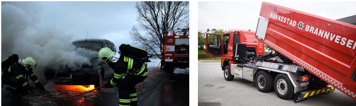
Figure 3-7: Conventional cooling of a battery pack mounted in the car's underbody [15] (left) and fire container of a Norwegian fire department [16] (right)
