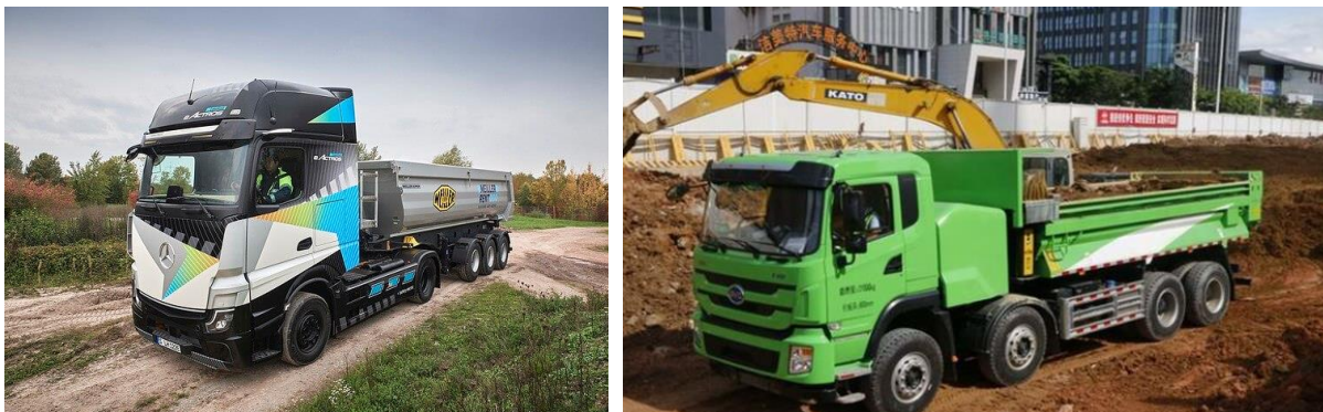
Figure 4-2: Examples of battery-electric trucks used in construction transport application from Mercedes Benz, showcase vehicle at the BAUMA 2022 (left) [26] and from BYD in 8X4 configuration (right) [28]
