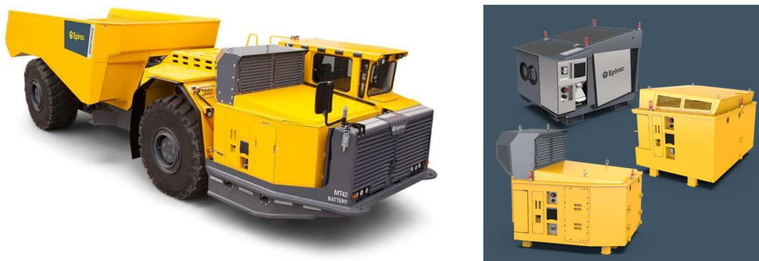
Figure 4-3: Epiroc battery-electric 40 ton ADT [36] (left) with examples of Epiroc battery packs [37] (right)
