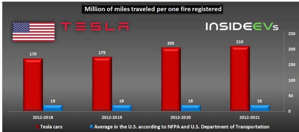
Figure 5-5: Comparison of vehicle fire probabilities for TESLA vehicles and average U.S. vehicles [58]
