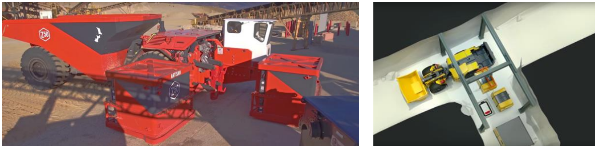
Figure 3-3: Examples of charging systems using battery swapping by a vehicle-based mechanism (left, source: Sandvik) and using an overhead crane (right, source: Epiroc)
