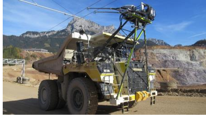
Figure 3-4: Examples of a trolley system already realised for road trucks (left, source: SCANIA CV AB) and for mining application (right, source: Liebherr [12])
