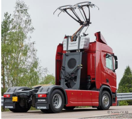
Figure 3-4: Examples of a trolley system already realised for road trucks (left, source: SCANIA CV AB) and for mining application (right, source: Liebherr [12])
