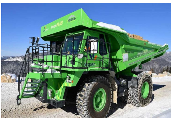
Figure 4-6: Kuhn / eMining prototype of a retrofitted Komatsu HD605-7 to battery-electric drive [52]
