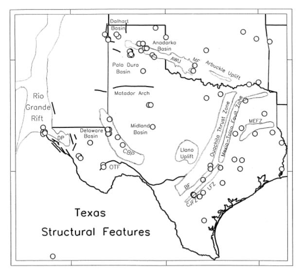
Figure 2. Structural features of Texas. Lines indicate faults and circles are where earthquakes were felt through 2001. The abbreviation AWU denotes the Amarillo-Wichita Uplift. From Frohlich and Davis (2002).
