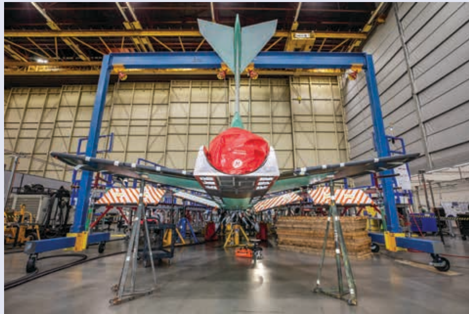
NASA's X-59 sits in support framing while undergoing the installation of its lower empennage, or tail section, at Lockheed Martin Skunk Works in Palmdale, California.
